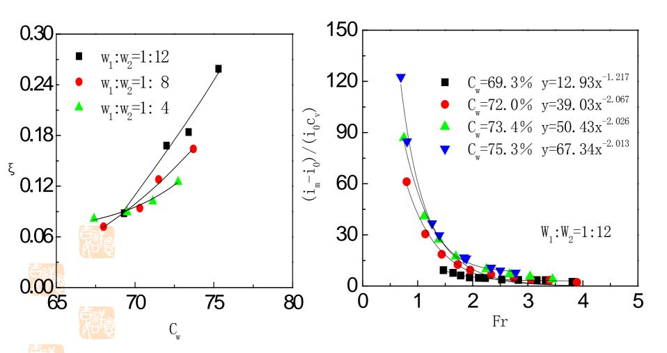
Fig. 2 The relationship between the resistance coefficient and concentration of the bending section
