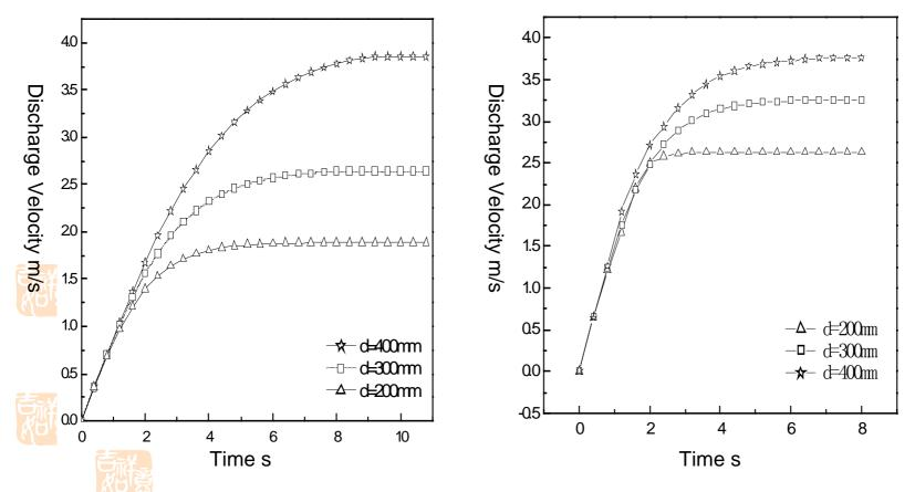
Fig 6 the relation between v~ t when  $c_v = 10\%$
